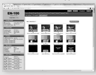
Adtec Digital has adopted zero-configuration networking technology, streamlining the setup and configuration processes for our products. The use of this technology enables automatic discovery of Adtec devices and services on an IP network. Used in tandem with the web-based control and configuration applications we can now provide 1-click access to any device.
