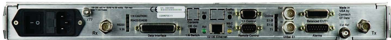
CDM-570/L-IP Satellite Modem back panel
