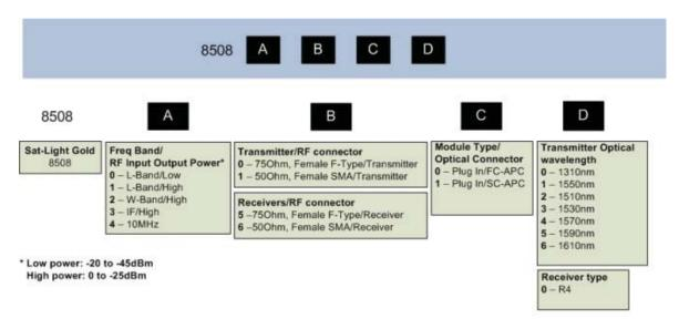
Example: Plug in module, L-band, low RF input, 1310nm laser, F-Type RF connector and FC/APC optical connector
