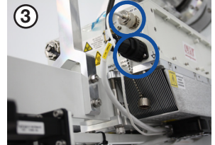
Connect cables(2EA) to the each connector on the right side of Ku-band BUC.
