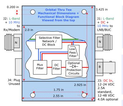
Standard Bias Tees are not designed for Satellite applications. They are very simple circuits, and will short the 10 MHz to ground:
