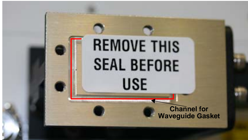
Figure 3.7 Waveguide Label and Channel for Gasket
