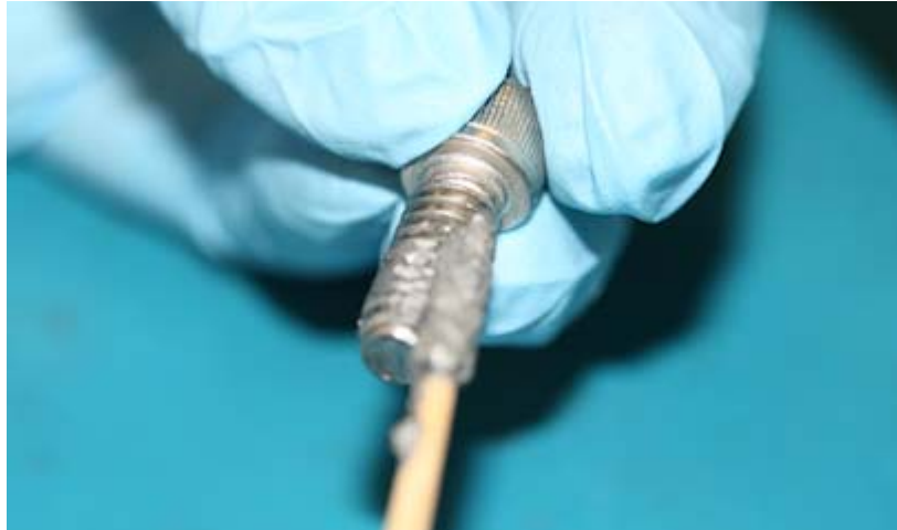
Figure 3.6 Applying the Anti-Seize Lubricant
