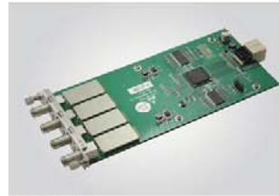
▶ DVB-T Receiver ▶ ISDB-T Receiver
