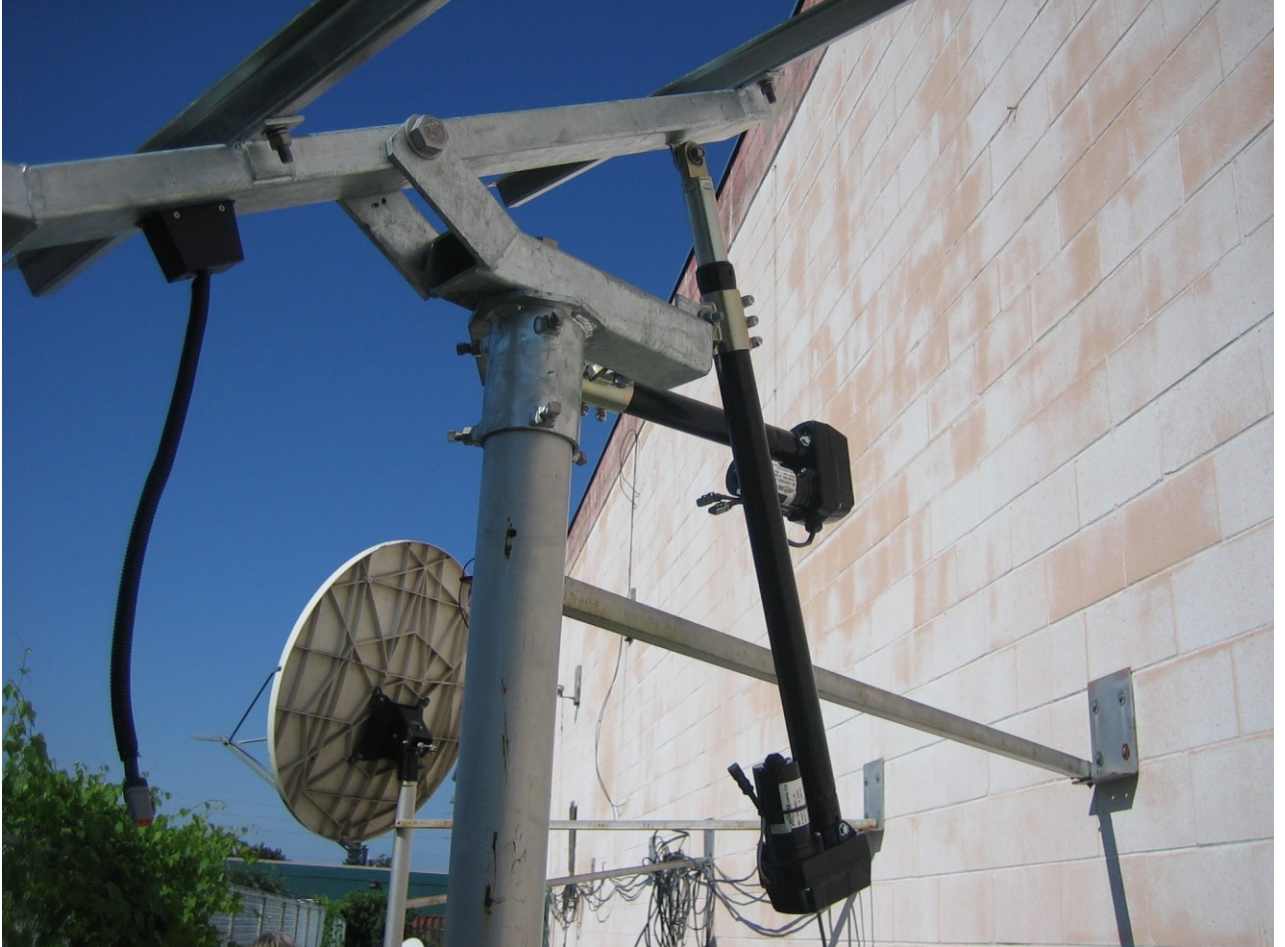
Fig. 3: Assembled Elevation Actuator
